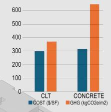
On carbon performance, the whole building (with 1-level concrete parkade and shaft) achieves a 30-35% reduction in embodied carbon compared to a full concrete baseline. Above grade, where mass timber displaces concrete, the reduction is more pronounced at 45-50%. Mass timber additionally acts as a carbon store, sequestering biogenic carbon for the life of the building. Optimized façades (~40% glazing) further reduce operational carbon by 10–15%, cutting long-term emissions.
