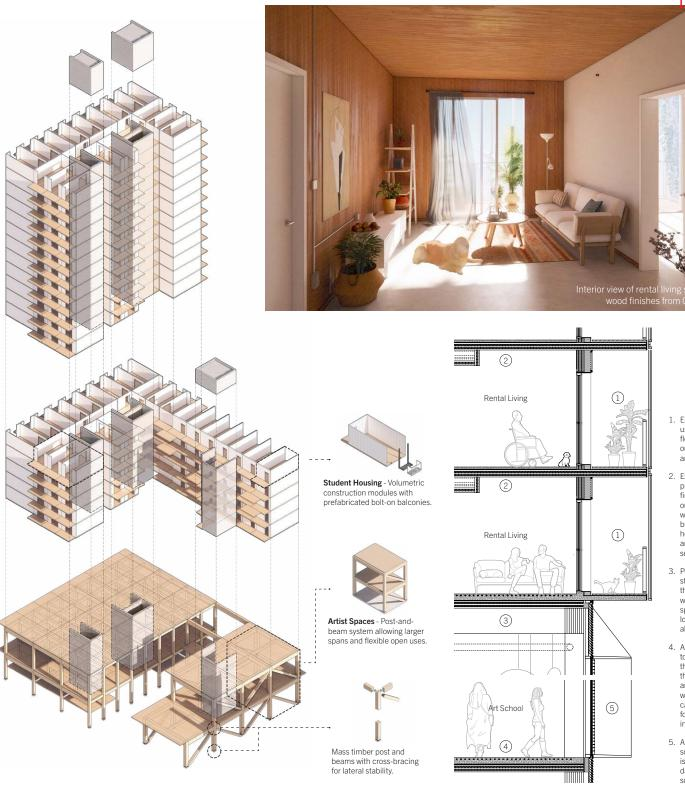
Enclosed balcony is used to protect CLT floor and provide usable outdoor space all year
