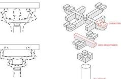
Schematic diagram of the abstract form of larger bracket as column capital replaced by interlocking self-similar smaller brackets to increase the stiffness as well as to transfer the roof and beam load sequentially to the column.
