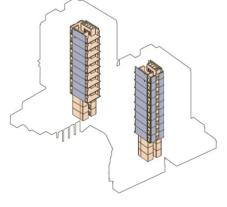
3. The infrastructural core rises within the tower, with 50 cm-thick concrete walls. In addition to elevators and the emergency stairwell, it also contains services wall and waste chutes.
