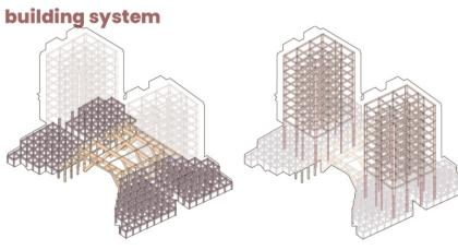
1. The communal market's structure 2. Above the public market, starting is lighter and more affordable, cutting construction costs and time. Structural modules measure 4x4x4 meters, half the size of tower modules.
