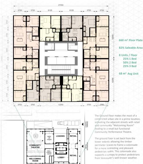
The units are based on a modular grid determined by the dimensions of a typical shipping tractor trailer. However, the design of the unit layouts goes beyond this utilitarian starting point with a focus on the occupants that will live in them.
