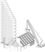
**VMUs** core, and corner 'starter' walls integrated CLT shear walls 'galleries' of corridors and posts offload lateral loads from the stack in a staggered solid/void complete the lateral forcemodules and counter story pattern. Shear walls run floor- resisting system by providing drift, diaphragm continuity, and to-floor to ensure continuous secondary vertical lateral paths.
