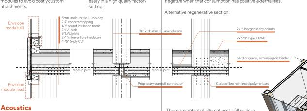
This proposal suggests a conventional assembly using 2.5" concrete topping to achieve both the encapsulation requirements and the acoustic requirements simultaneously. However, the concrete topping in this floor assembly has by far the highest global
