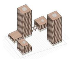
We employ a hybrid timber structure-mass timber columns and beams with CLT floor panels-to reduce embodied carbon, paired with a concrete core to meet BC Building Code requirements for fire protection and seismic performance.
