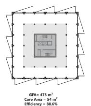
The open structural grid supports highly adaptable layouts. By concentrating services within the first bay, the remaining unit space enjoys taller ceilings and a more generous interior atmosphere. With a compact core and a floorplate efficiency of 88.6%, the design maximizes usable area—supporting affordability, flexibility, and future-proof planning.
