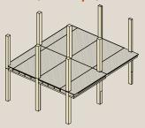
Structure is comprised of GLT columns and CLT slabs which will form a ribbed cassette once the interior module is placed.
