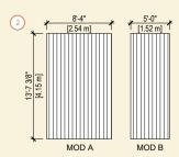
Maximum dimensions of modules in BC without requiring permit or pilot car for transport are 8'6" x 53'-0".
