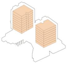
4. A total of nine residential floors are built. The rooftop level will be used for the installation of solar panels, water tanks, and service equipment.
