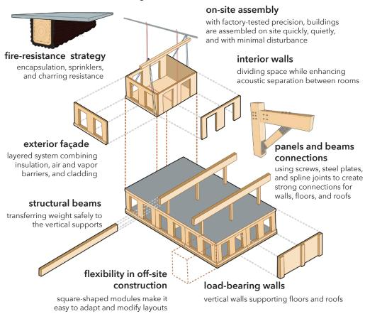
Mass timber buildings require protected connectors, durable envelopes, and careful detailing to meet safety and energy codes. This includes ensuring fire protection, weather resistance, and acoustic performance, while also addressing challenges like shrinkage, wood variability, and thermal bridging to deliver safe, efficient, and long-lasting multi-storey construction.
